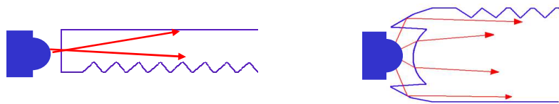
Fig.2 Example of light coupling from LED.
