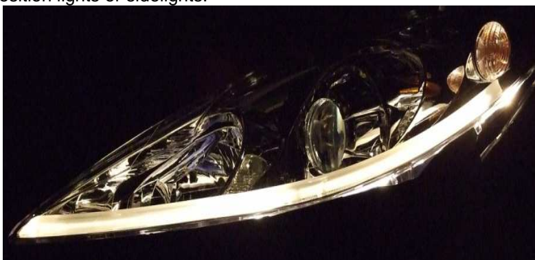
Design study of headlamp equipped by light guide to increase the bottom edge of headlamp.
